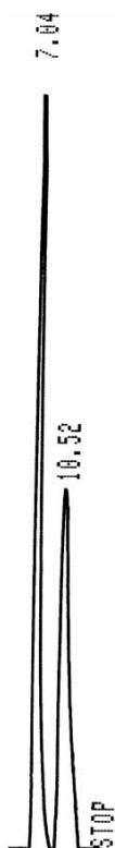
Figure 6. A chromatogram of separation of the hexabenzylidigerinoxane (7.04 min) and hexabenzylidigermanium (10.52 min) on the stationary RP Si-PGC phase. Mobile phase: acetonitrile/water (80/20 vol.%); flow -0.3 \text{ mL} \cdot \text{min}^{-1} , wavelength -242 \text{ nm} , temperature -20^\circ\text{C} .
